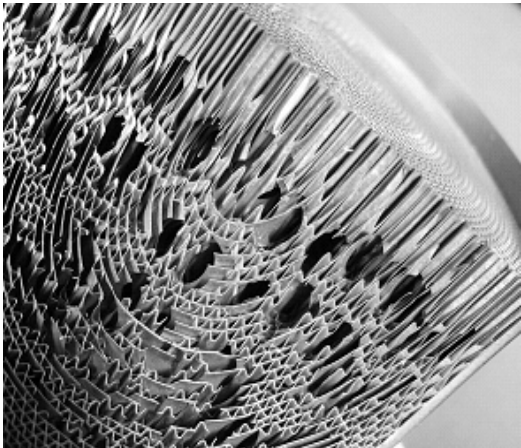
Figure 11: Cut of a PE Metalit®
