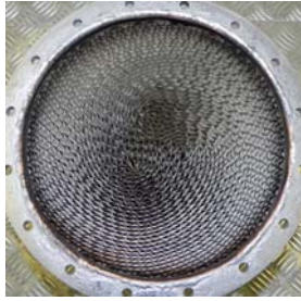
Figure 19 H-Cat: no deposit after 10 h @ A 25 load point
