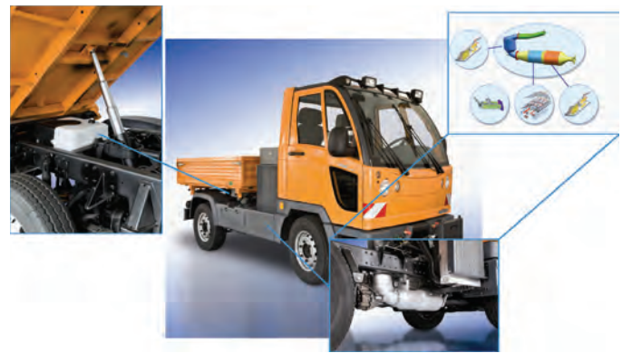
Figure 16. The Multicar Test Vehicle Including the Installation of the SCRi ® Catalyst System and the SCR Dosing System Under the Loading Area for Retrofit [21]
