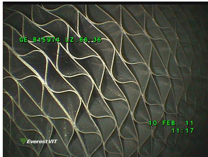
Figure 5 – Gas inlet face of the substrate with 1.5mm Standard mantle at 66hrs of the accelerated thermo-mechanical test.
