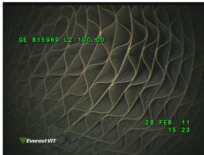
Figure 6 – Gas inlet face of the substrate with 0.5mm Vault-structured mantle at 100hrs of the accelerated thermo-mechanical test.
