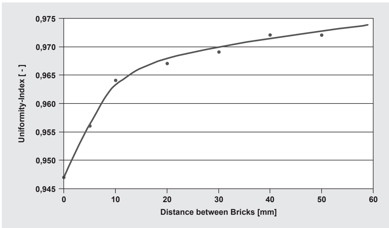
Figure 3: Uniformity index as a function of the gap between the two substrate halves (massflow 444 kg/h; room temperature; catalyst \varnothing 93 x 78 mm/600 cpsi/40 \mu m uncoated)
