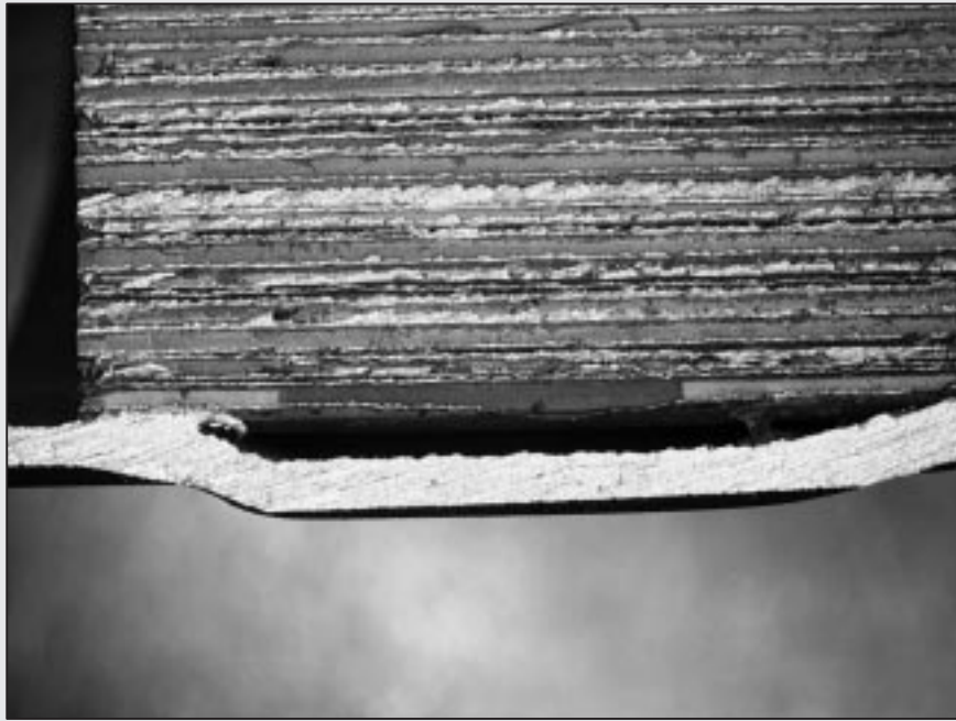
Figure 4: Sectional view of the hybrid catalyst with air-gap insulation on the gas inlet zone
