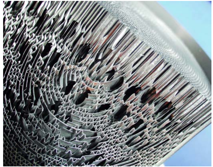
Fig. 2: The structure of PE substrate with the formation of cavities
