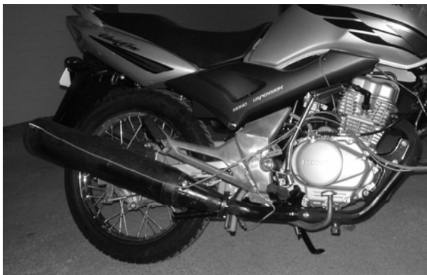
Figure 5. Exhaust system setup on tested vehicle.
